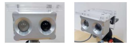
The sensor is sensitive for fog particles in a zone about 10 to 20 cm ahead of the location of the sensor who limit the visibility in the air. These particles are normally the microscopic water particles constituting fog, but they may also be snowflakes, raindrops or air pollutants. But the most indications of low visibility are because of fog or snow.
