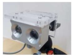
The sensor is heated to a few degrees above ambient temperature in order to keep moisture away. In order to keep the electronics dry a membrane ventilator that keeps the pressure inside at the same level as outside. This prevents liquid water from sucking into the sensor through micro cracks etc. at falling temperature – a creative solution to a big problem.
