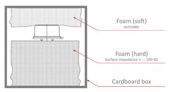
This packing is used for classic ESD protection. Otherwise, it also protects against inherent risks of pyroelectric detectors. A pyroelectric sensor element can generate a voltage of 1 kV if exposed to a temperature difference of some 10 K. In the case of an open connection configuration, which is often used for current mode detectors, high
