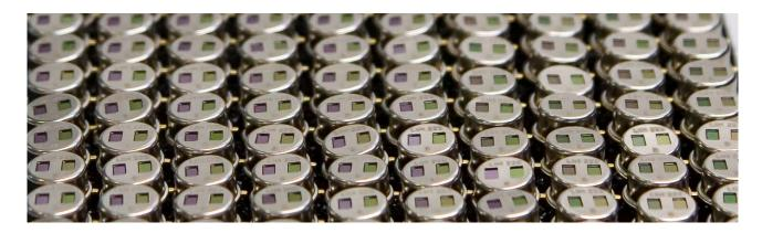
Our products comply with the normal requirements for electronic components regarding transportation and storage. Protect the components especially against exceptional mechanical loads or harmful, particularly corrosive gases or vapors. The storage temperature limits specified in the data sheets must not be exceeded.
