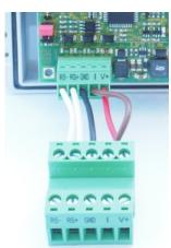
Cables with a cross-section up to a maximum of  $2.5 \text{ mm}^2$  single-wire or  $1.5 \text{ mm}^2$  strand such as LiYCY  $3 \times 1.5 \text{ mm}^2$  can be connected via the adapter plug supplied.
