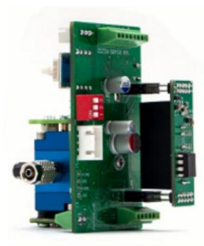
Figure 5 Flow EVO plus Type II with isolated analog interface
