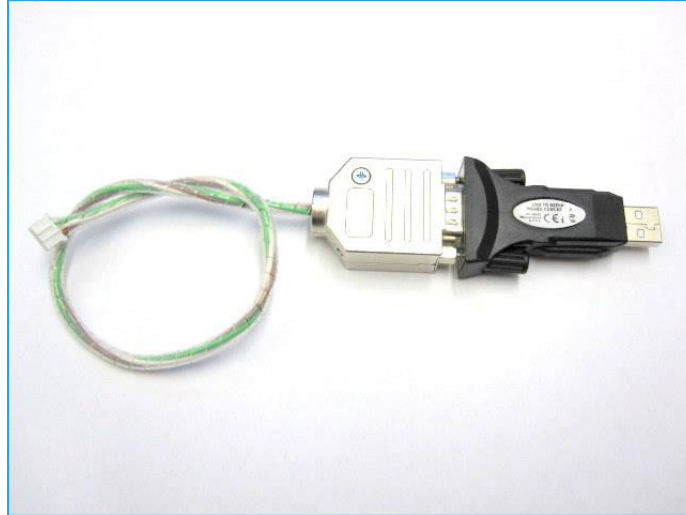
Figure 2: USB adapter for operating a BASIC EVO on a PC
