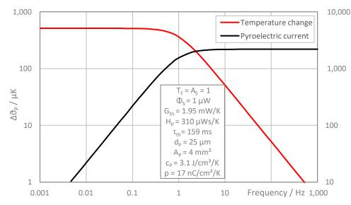
Figure 3: Frequency dependence of the temperature change and short-circuit current of a pyroelectric element
