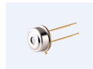
The OTP-N537F2 is a thermopile sensor in classic TO-5 housing. The sensor is composed of 116 elements of thermocouple in series on a floating micro-membrane having an active area of diameter 545  $\mu\text{m}$ . The thermopile sensor provides nearly Johnson-noise-limited performance, which can be calculated by its ohmic series resistance. A thermistor with a lead connected to ground is also provided inside the TO package for ambient temperature reference.
